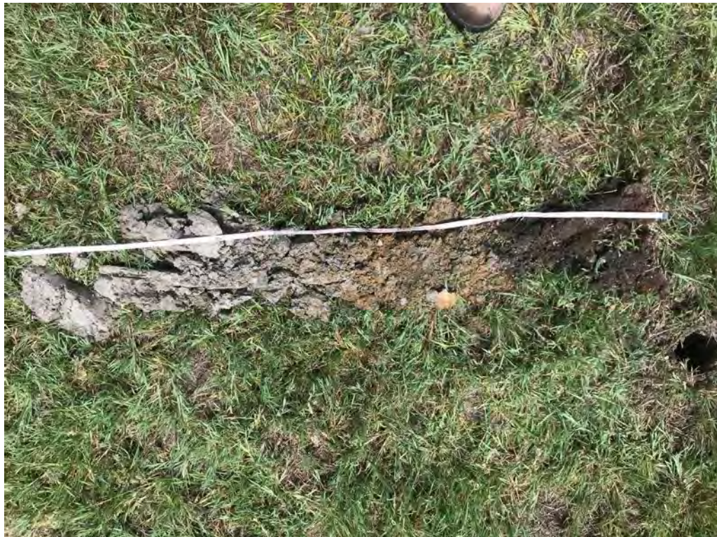
Photo 10: View of soil profile from augured observation pit #2. This pit was located towards the center of the field. Hydric soil indicators were observed within 12" of the soil surface and the water table was measured at 16" below the soil surface.
